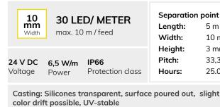
Separation point 167 mm Length: 5 m Width: 10 mm Height: 3 mm Pitch: 33,33 mm 25.000 h L70 | B10 Hours:
