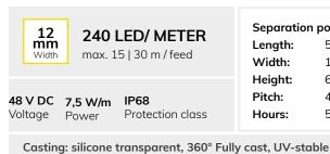
Separation point 50 mm Length: 5/30 m Width: 12 mm Height: 6 mm Pitch: 4.16 mm Hours: 50.000 h L70 | B10
